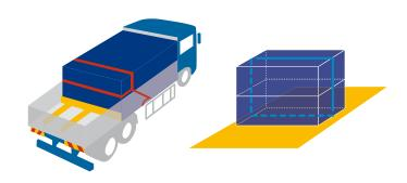
If the cargo is equipped with lashing eyes compatible with the strength of the lashing, it is possible to lash directly between the lashing eyes and the lashing points on the vehicle.
