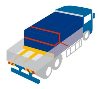
Vertical round turn cargo lashing is used to bind a number of cargo items together to stabilise the cargo section and to increase vertical pressure between the layers. Risks of internal sliding are thus reduced.
